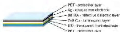
Fig. 1. Schematic diagram of an electroluminescent lamp.
