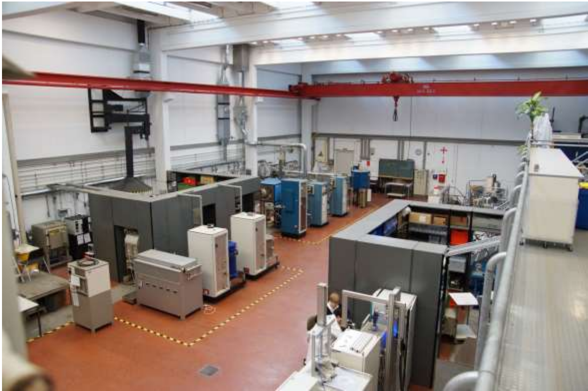
Technical hall (600 m 2 ): equipped with facilities for advanced processing, shaping, melting, and sintering as well as molding of glass, ceramics and composites
